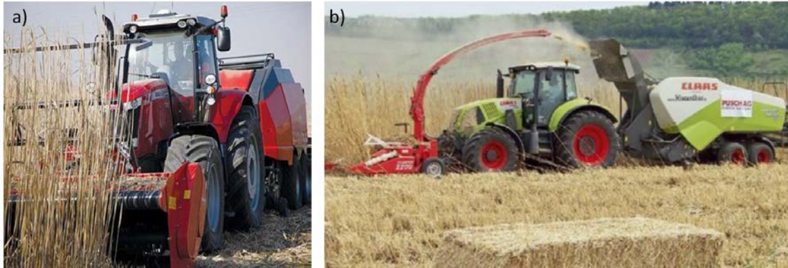
Figure 5. a) Single passage harvesting and baling with front shredder and baler. b) Production of chopped and baled biomass with forage harvester and modified baler. Both photos are taken from [10].
