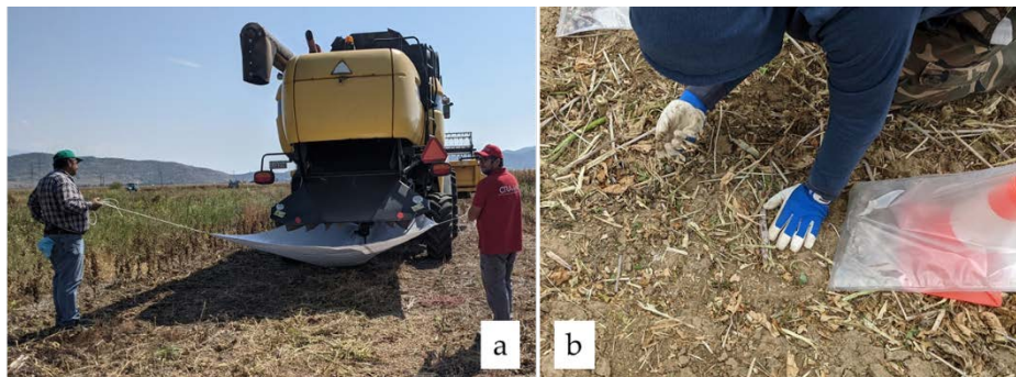
Figure 13. Collection of threshed biomass (a) and lost capsule (b) for CSL and ISL assessment respectively.
