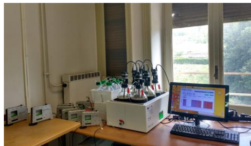
Fig.1 AMPTS, Automatic Methane Potential Test System
